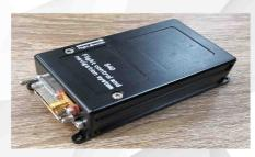
S40 is the full autonomous flight controller and navigation system specifically designed for compound UAVs VTOL (vertical takeoff and landing fixed wing), which is also suitable for an air with the conventional fixed wing+quadrotor configuration. It internally integrates the flight control computer and micro-assembly navigation system (GPS/INS). Simply one-key action, it is capable of enabling automatic
